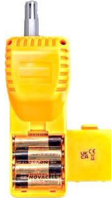
Figure 2. Installing the device power source - batteries
